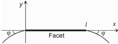
Figure 1 Geometry of a facet (bold line) connected with non-singular GBs at sharp edges.
